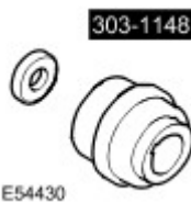
Installer oil seal front cover 303-1148
