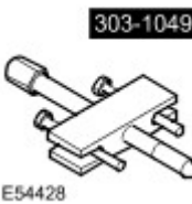
Remover crankshaft damper pulley 303-1049
